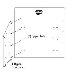
Align Part #3 upper left side and Part #6 upper back using 4 pan head screws.
