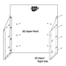
Repeat the same process align Part #4 upper right side to Part #6 upper back using 4 pan head screws.
