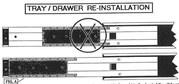
When re-installing tray(s), the ball bearing retainers must be brought to the front of the slide on left and right slides to ensure safe re-installation as shown in FIG. A. At this point, align slides on tray and gently push in until tray slide snaps into lock position.
