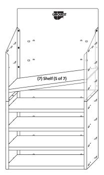
Place Part #7 shelf into the bottom row of shelf supports, by placing on an angle as shown, lift right side above support clips and push down. Make sure the shelf is secured in all six support clips.
