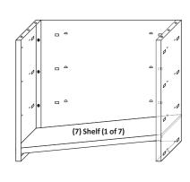
Begin by locating Part #1 lower left side and Part #5 lower back. Align the machined holes making sure the **shelf support clips are facing up**. Locate the weld nuts on Part #1 lower left side, secure Part #5 lower back using 4 pan head screws.
