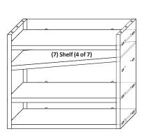
Place second shelf onto the top row of shelf support clips. This should be done on an angle, same as the previous step.
